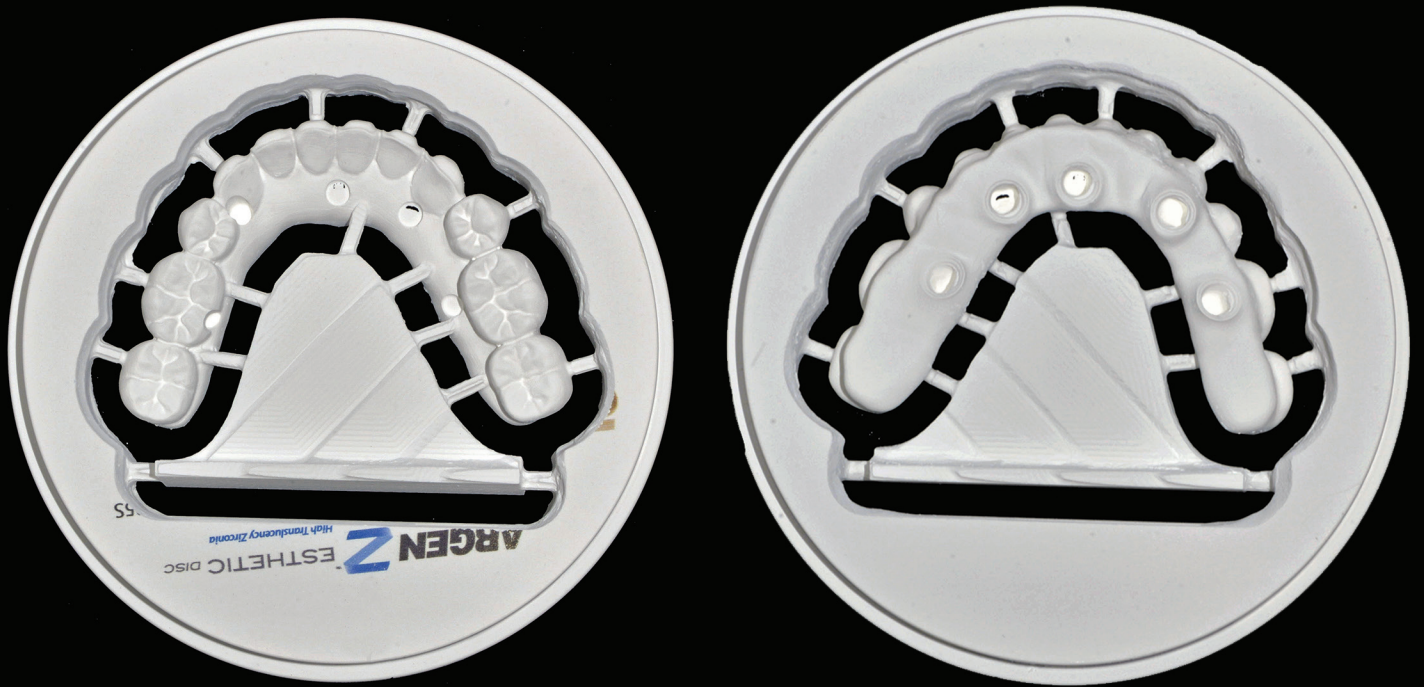
Figure 12. Full arch prosthesis after being milled prior to sintering
