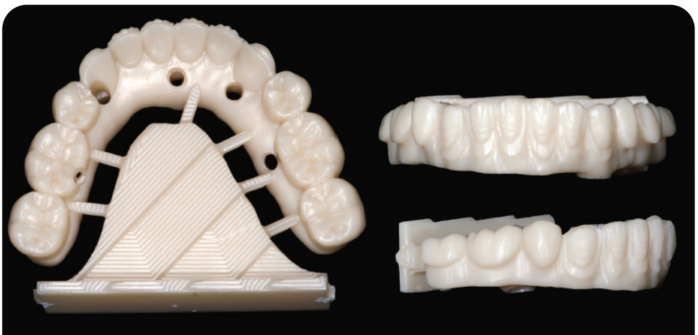
Figure 13. Zirconia restoration after being sintered
